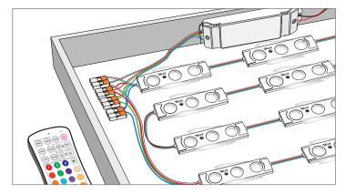
Wire both ends of LED modules to the controller and power supply. For multiple series, connect them in parallel to avoid voltage drop (refer to page 2).
