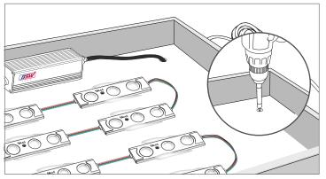
**6** Drill holes along the edge of the channel letter or lightbox connect to the power.
