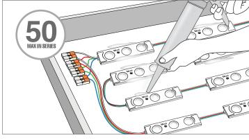
**4** WAGO connectors enable quick wiring of LEDs in series and ensure the correct polarity with white (+), R + R, G + G, and B + B. Secure the LEDs using silicone glue.
