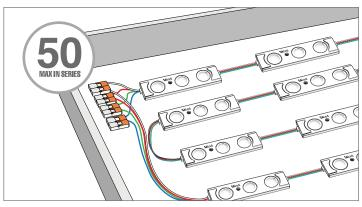
**3** Ensure modules are connected in series or parallel (refer to Figure 2 on page 2). Avoid exceeding the maximum module count to prevent voltage drops.
